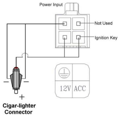
In the above diagram, pin 1 is connected to the Cigar-lighter Connector minus, and pins 3 and 4 are connected together to the Cigar-lighter Connector plus.
