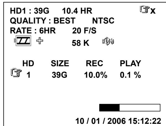
**(HD1: 39G):** Total capacity of installed hard disk, 39 GB.
