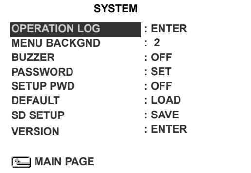
This page is used for accessing the history of the operation status, setting the password, resuming factory default, and determining the menu display background.
