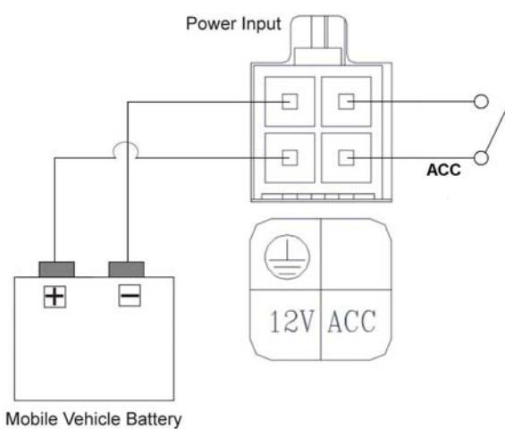
In the above diagram, pin 1 is connected to the vehicle battery minus, pin 3 to the battery plus, and pin 4 to the vehicle ignition key.
