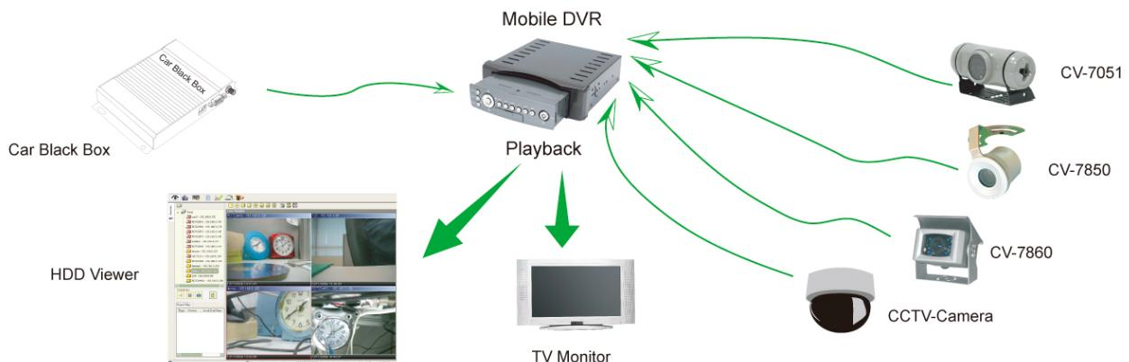
The mobile DVR is compatible with the stand-alone GPS receiver, and it can also configure and record a driver's location (latitude and longitude) with video data. Besides, it can playback video by our HDD viewer software, which can track a driven route using all GIS/e-Map software.
