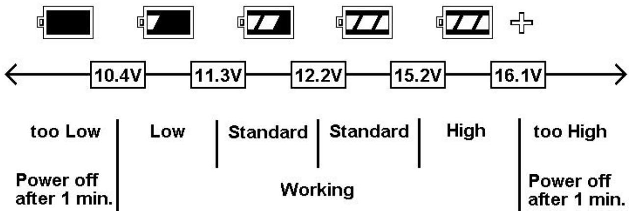
You can display the system - setting information after you press the "DISPLAY" button on the front panel. On this screen you can see the battery voltage icons. Please consult the above diagram to know the battery voltage status.
