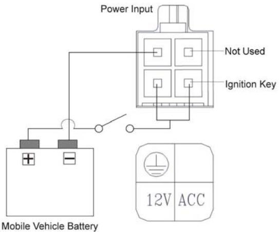
In the above diagram, pin 1 is connected to the vehicle battery minus, and pins 3 and 4 are connected together to the vehicle battery plus.
